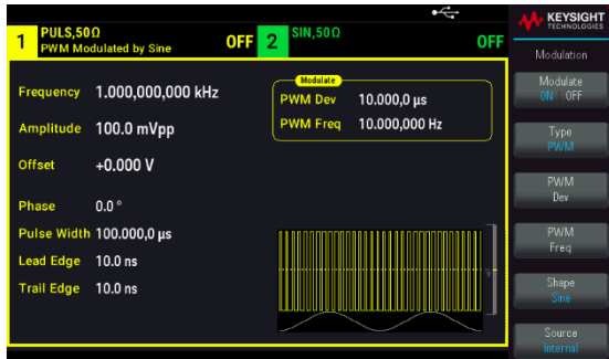
Figure 3. PWM modulated with standard sine wave
