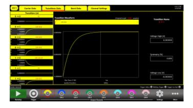
The software architecture provides the possibility to easily generate the patterns in different generation modality and also gives the opportunity to modulate the patterns with internal or external signals with the purpose to generate also different effects of noise (jitter, ripple, ...).
